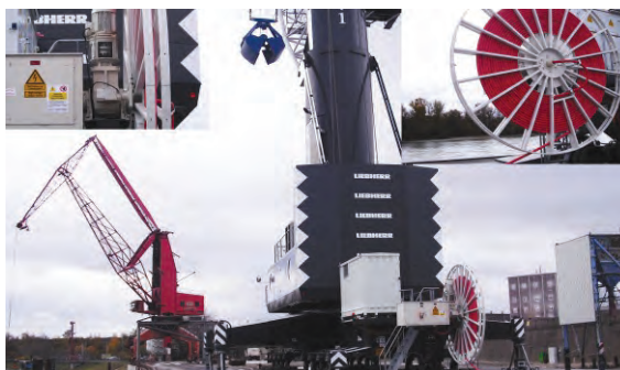
Mono spiral cable reeling drum on a large Liebherr mobile crane.
