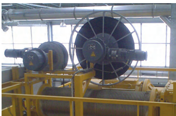
Mono spiral and cylindrical motor driven drums paying vertically down to hook on a special overhead crane.
