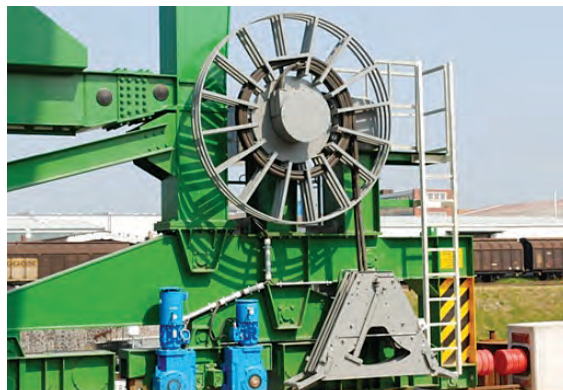
Twin cable spiral cable drum on large gantry crane.
